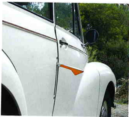
Trafficators – the fiddly little pretend hand, which swings out from the car in imitation of a hand signal – followed familiar products and practices.
